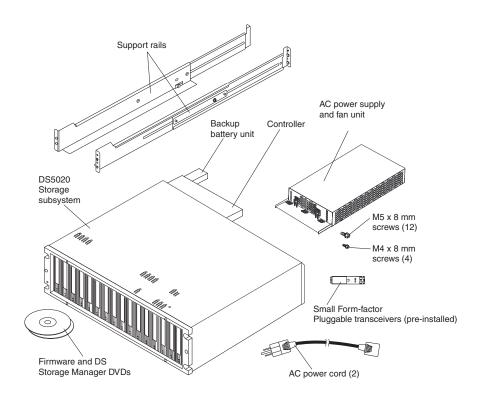
Complete the following steps to prepare the DS5020 storage subsystem for installation into a rack cabinet:
